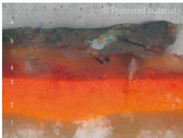
8. Anonymous, Catalan The Majesty of Christ on the Cross Bilbao Fine Arts Museum Stratigraphy of a sample taken from grey on red in a rhombus of Cross decoration (MPlan 20 X / 0.40 kens) 1. White gypsum and silicate ground (v. l. p.) (350 µm) 2. Orange comprising white lead, vermilion (l. p.) and calcium carbonate (l. p.) (25 µm) 3. Red comprising vermilion, white lead and calcium carbonate (v. l. p.) (15 µm) 4. Red comprising red colouring, white lead (l. p.), calcium carbonate (l. p.) and vermilion (35-40 µm) 5. Grey-brown, tin adhesive (20 µm) 6. Tin-plate silvering (25 µm)
