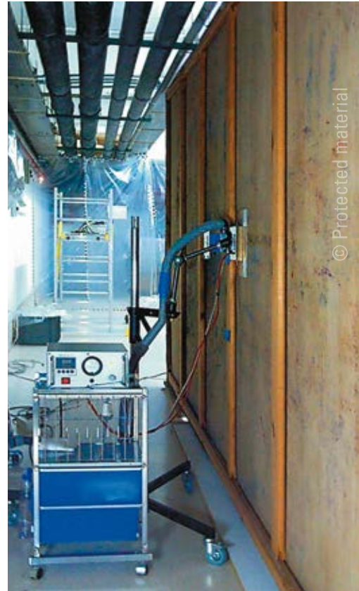
10. Mitka low-pressure mini-table working on the reverse of Big Garden
